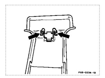
Retaining clip at top in B-pillar panelling
