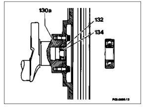
Radial ball bearing (134) and locking ring (132)
