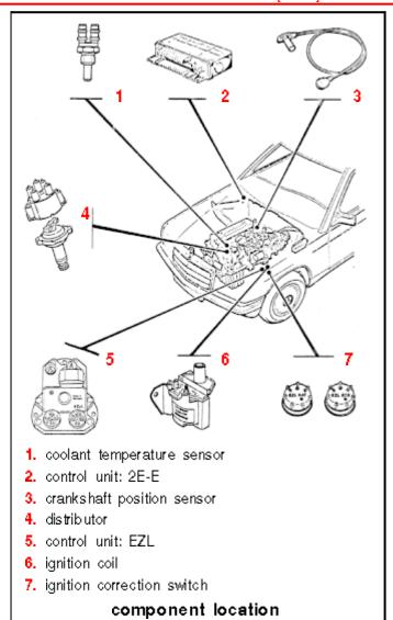
This is an electronically controlled ignition with a control unit and diagnostic connector.
