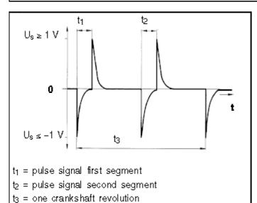
signal crankshaft position sensor
